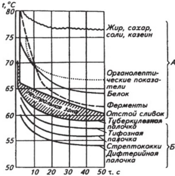
Fig. 1. The dependence of the pasteurization temperature on the duration of exposure
